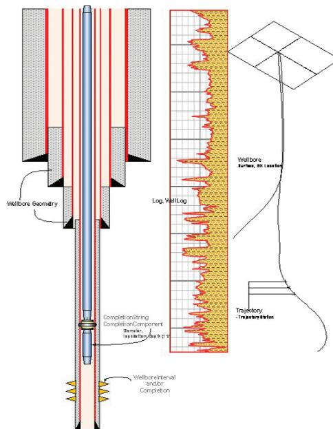
*RESQML integrates with companion XML-based standard WITSML to use these well-related components. (Figures courtesy of Energetics)*
